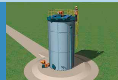
ZipaTank™ is manufactured to API 650 or BS 2654 standards
